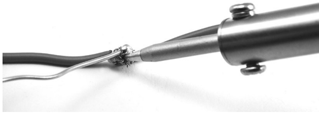
FIGURE B-4: RUNNING SOLDER INTO THE JOINED WIRES
