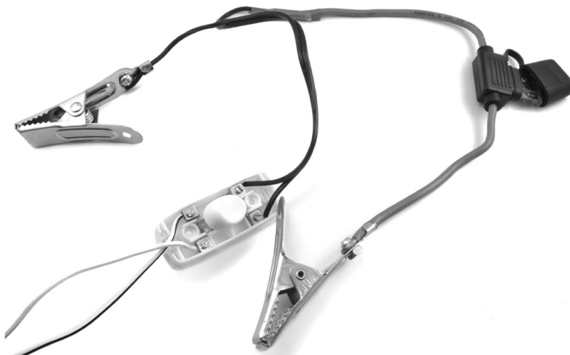
FIGURE 3-7: CONNECTING THE FUSE AND ALLIGATOR CLIP FOR A LIGHTING SYSTEM
