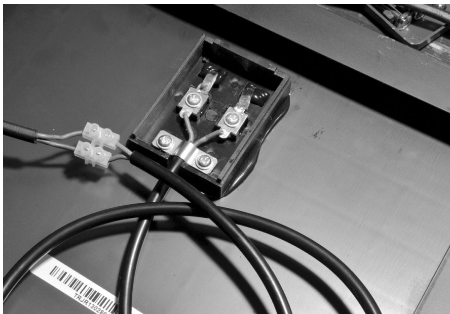
FIGURE 2-7: CONNECTING THE SOLAR PANEL
