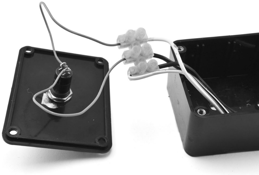
FIGURE 6-9: WIRING UP THE SWITCH BOX
