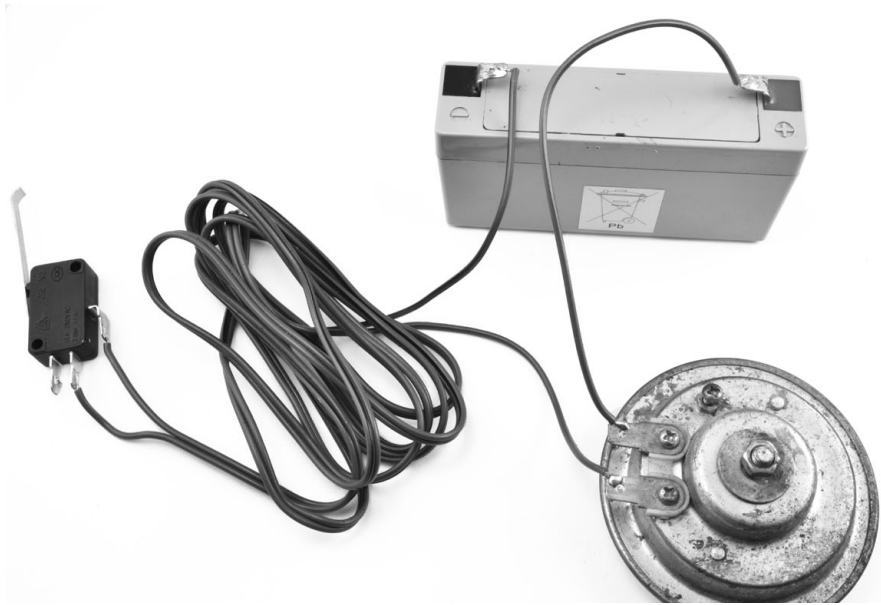
FIGURE 4-8: THE FINISHED WIRING
