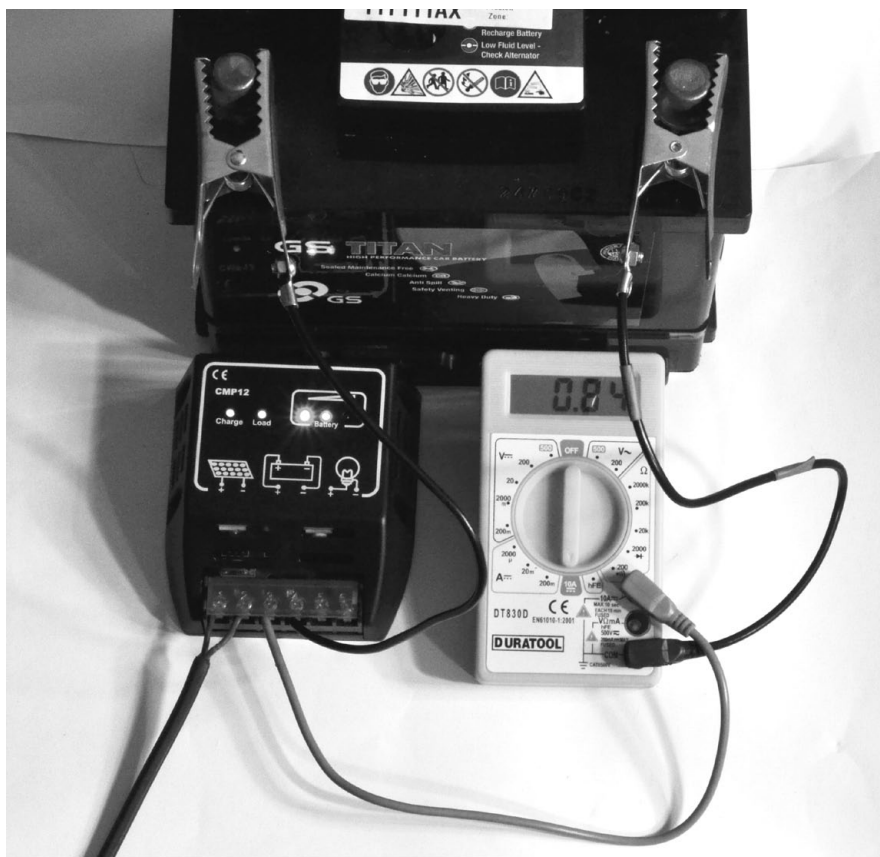
FIGURE 2-11: THE CHARGE CONTROLLER, MULTIMETER, AND BATTERY ARE CONNECTED.
