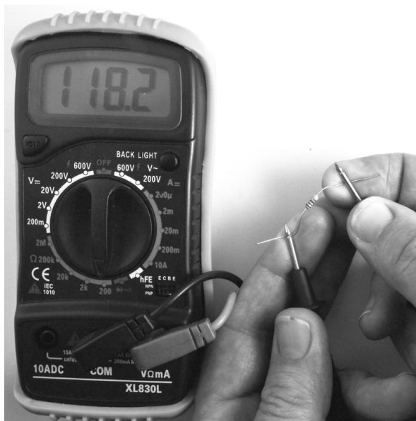
FIGURE B-13: MEASURING RESISTANCE WITH A MULTIMETER
