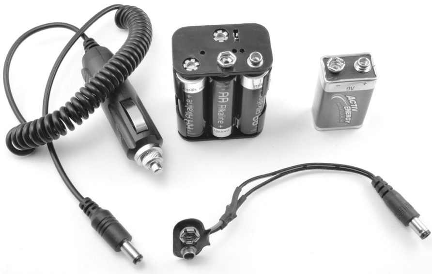
FIGURE 9-10: OPTIONS FOR POWERING THE ARDUINO
