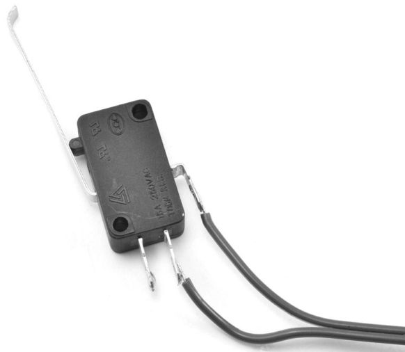
FIGURE 4-7: SOLDERING WIRES TO THE SWITCH
