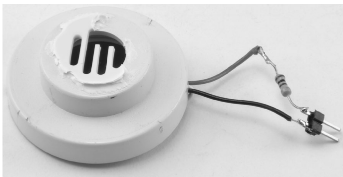
FIGURE 9-14: SOLDERING THE BUZZER, RESISTOR, AND HEADER PINS
